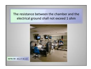
Class B chambers with>23.5% O2: Electrical grounding of the patient shall be ensured by the provision of high impedance conductive pathway in contact with the patient's skin.
